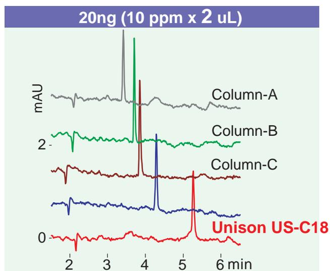
Large injection volumes are required for trace analysis. ODS columns can be overloaded (resulting in peak splitting / loss in retention) when a large volume of a strong solvent (ACN) is injected into a weak eluent + ODS column. Reducing the injection volume minimizes this effect - but results in a loss in sensitivity.
