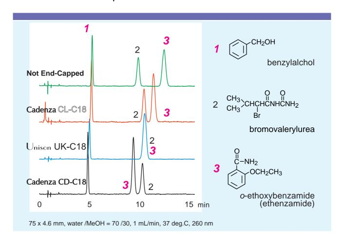
In addition to hydrophobic interaction, several secondary interactions occur within an ODS column. For example, silanols or siloxanes from the surface of silica can also interact with certain analytes (electrostatic interaction). Many compounds are affected by this secondary interaction.
