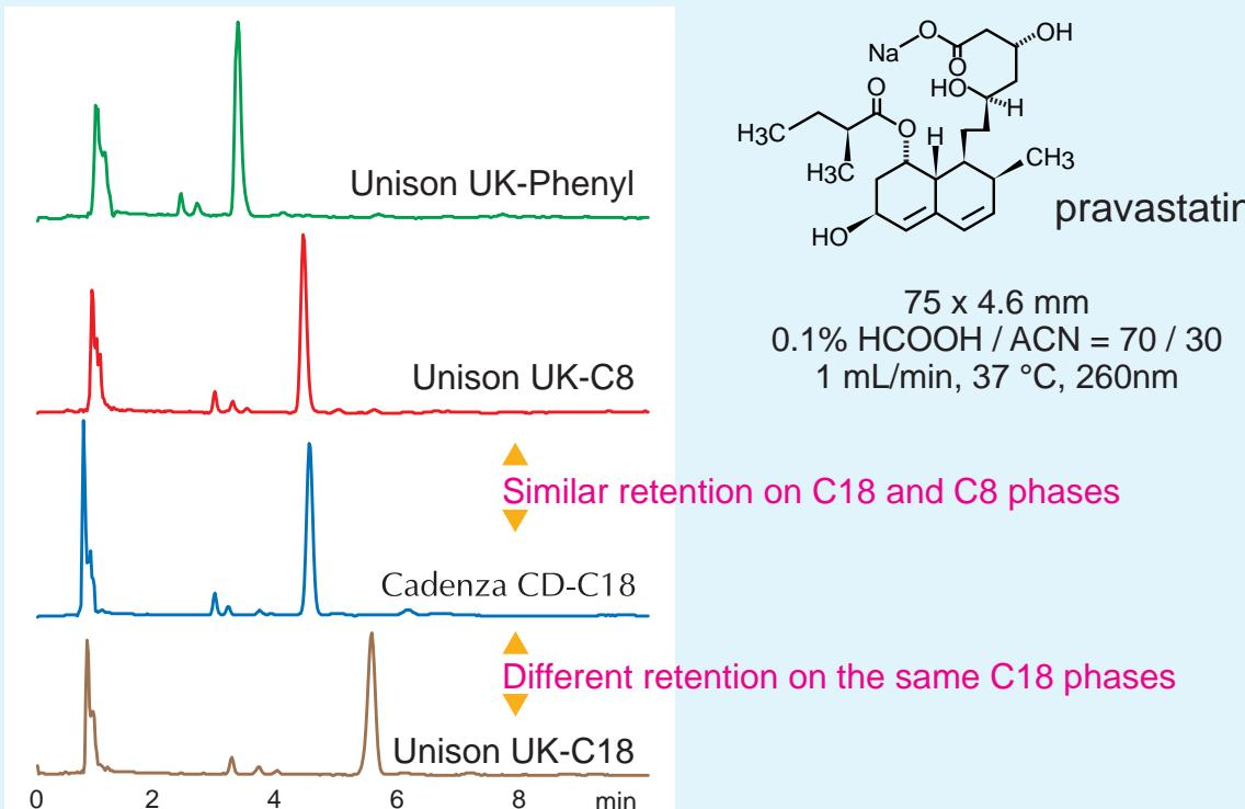
Unison series are compatible with 100% of aqueous eluent, and designed to provide better retention and separation for hydrophilic compounds. In contrast, Cadenza CD-C18 phase is designed with high ODS density to achieve better molecular recognition due to large steric selectivity.
