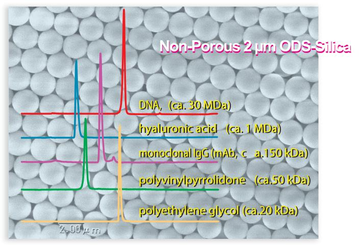
Imtakt has developed a novel 2um non-porous high resolution ODS column.
