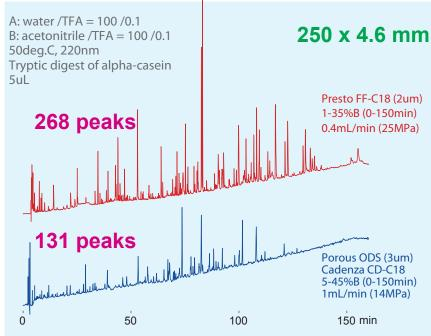
Presto FF-C18 enables unbelievable separation power for peptide mapping. Accurate trace analysis for peptides is very important for proteome analysis, but can be compromised with porous ODS column - due to adsorption in micro-pores.
